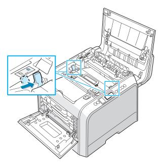
**15** After making sure that the left cover is open, close the top cover. Make sure that it is securely latched.
